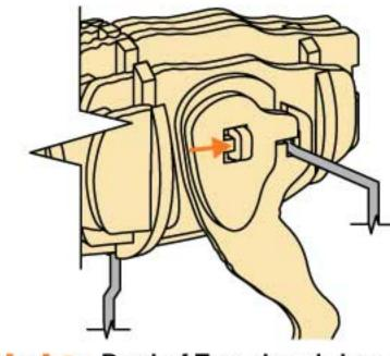
Note: Push 4E to the right until the notch slides into the space on piece 3F and locks in place.
