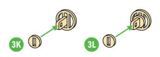
**Note:** Pieces **3K** and **3L** are designed to rest loosely on piece **3H**. This is to allow the legs to move back and forth. Steps in the following section will secure these pieces and prevent them from falling out.
