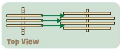
**Note:** Slide the neck pieces into the head pieces as shown in the "Top View" image above. Make sure the holes in the neck and head pieces are aligned so **2I** can slide all the way in.
