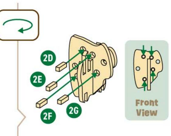
Note: Pegs 2D, 2E, 2F, and 2G are designed to rest loosely in the slots in 2B. This is to allow the torso to move while remaining structurally sound. The following step will secure these pieces and prevent them from falling out.
