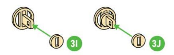
**Note:** Pieces **3I** and **3J** are designed to rest loosely on piece **3F**. This is to allow the legs to move back and forth. Steps in the following section will secure these pieces and prevent them from falling out.
