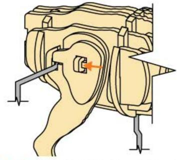
Note: Push 4B to the left until the notch slides into the space on piece 3H and locks in place.
