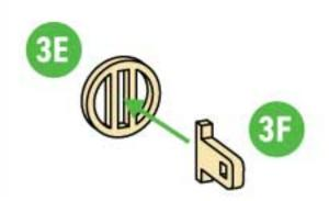
Note: The flat end of piece 3F should rest flush with the back of piece 3E.
